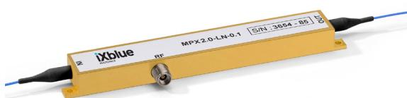
The MPX2000 and MPZ2000 are phase modulators specially designed for phase modulation in the 2.0 μm wavelength band from low frequencies to 10 GHz and above. The MPX/MPZ2000 incorporate 2.0 μm specific waveguides and are pigtailed with 2.0 μm polarization maintaining fibers.
